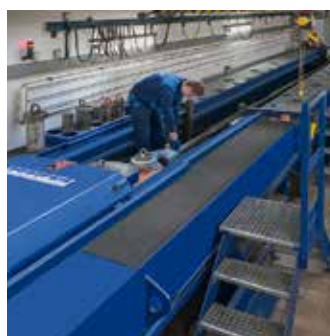
Pull Test Facility 6,000 kN
