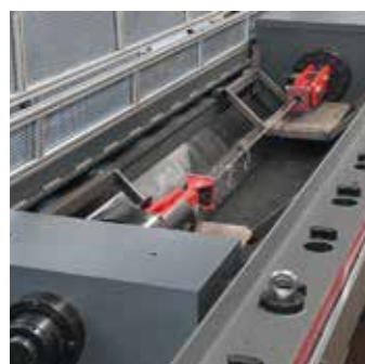
Pull Test Facility 800 kN
