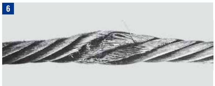
Bend caused by a pinched rope sling
