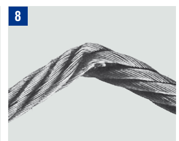
Kind caused by mechanical impact
