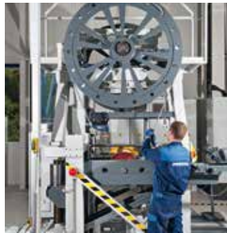
Test Facility for Determining Bending Fatigue
