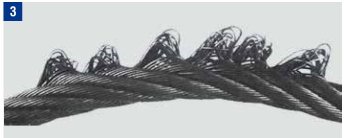
Through corrosion and wear heavy loose strand
