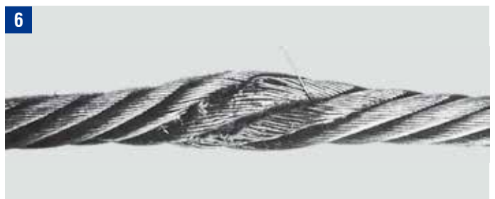
Bend caused by a pinched rope sling
