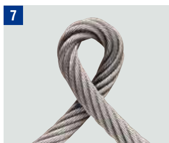
Bend caused by a pinched rope sling
