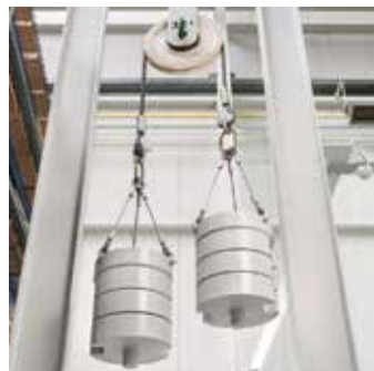
Rope Efficiency Test Facility
