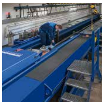
Pull Test Facility 6,000 kN
