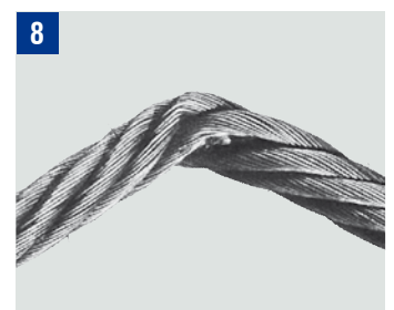
Kind caused by mechanical impact
