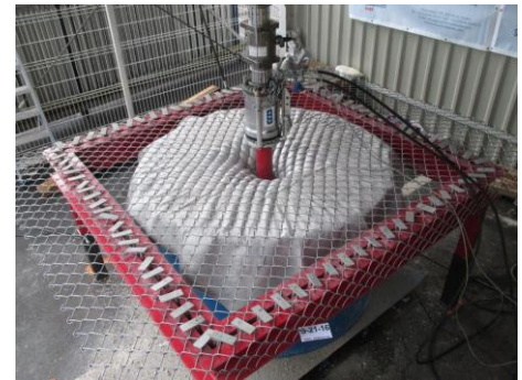
Puncture strength test under "supported" conditions.
