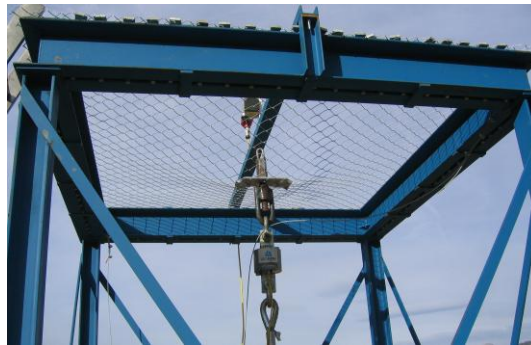
Puncture strength test under "open-air" conditions.
